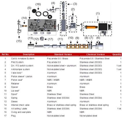
Note (\*): Items marked with an asterisk require thin film of lubricant.
