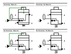
Emergency Shut Down with Easytork Solenoid Valve
