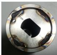
Drive insert welded into extended lower shaft
