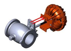
When installing the actuator to the valve, the shaft slot on the actuator must indicate the valve axis at the time of assembly.
