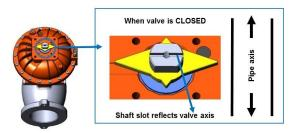
NTV governs the fail-safe action of the actuator, refer to NTV IOM for specifics on NTV mounting style. Not installing the NTV allows for double-acting setup. The mounting style of the NTV governs the fail-safe action of the actuator.
