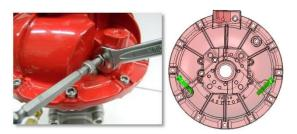
The rotation of the control valve package is to be stopped by the actuator's stopper bolt, and not on the stops on the valve. Failure of using the actuator's travel stop may 1. Possibly compromise the valve if "Valve MAST & Max Allowed Air Supply to Actuator" is not adhered to 2. Possibly result in damage to the actuator and will void Easytork's warranty and liability.
