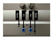
Port 2 and 4 are NAMUR standards. Pressure entering port 4 rotates the actuator clockwise, and pressure entering port 2 rotates the actuator counter-clockwise. The **Nest** ports interface the air reservoir.
