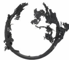
Vacuumed environment damages actuator soft sealing
