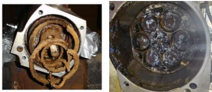
Actuator breathes in and out the environment in spring-return
