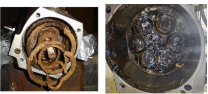
Actuator breathes in and out the environment in spring-return
